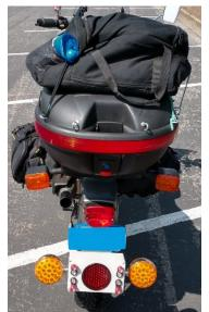
running them in phase with the stock signals. This is a Good Thing, because using them at full brightness tended to make the brake and tail lights much less noticeable.
